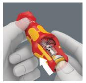
The Turbo function can either be switched on or off by pressing a button. For initial loosening and final tightening at increasing torque moments (or fine torque adjustment) of screws the Turbo function is disabled. For free running screws the Turbo function is enabled.
