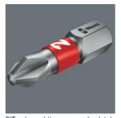
BiTorsion bits are absolutely premium products. They have a softer BiTorsion zone which reduces the hardness of the shaft by about 20 % in comparison to the drive tip. This means that the peak loads that cause bit breakage and premature wear are absorbed in this zone — something which enhances the service life of the
