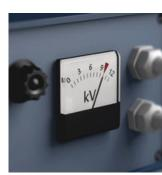
The individual testing at 10,000 volts, in accordance with IEC 60900, ensures safe working with loads up to 1,000 volts.
