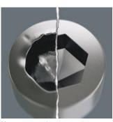
Hexagon socket screws are a problem, because the contact surfaces that transfer the force of the tool to the screw are very narrow. The consequence: the head of the screw can be damaged, usually rounding out the recess. Hex-Plus tools have larger contact surfaces to prevent this, driving from the flats of the recess, rather than the corners. Good to know: Hex-Plus tools fit into every standard hexagon socket screw!
