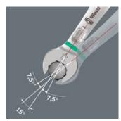
Thanks to the mouth side pivoted by 7.5°, double hexagon geometry and an adjusted application method (placement – screwdriving – turning – replacement – screwdriving – turning, etc), even screwdriving challenges allowing a pivoting angle of less than 30° can be solved.
