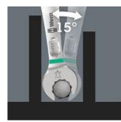
The Joker 6003 combination wrench with its special mouth geometry – an open-end offset by 7.5° and the double hexagon geometry – doubles the placement possibilities when repeatedly turning the wrench 180° around the longitudinal axis. Bolts and screw heads can be "accessed" every 15°. The Joker 6003 will automatically find the respective placement point after every turn.
