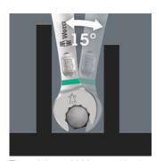
The Joker 6003 combination wrench with its special mouth geometry — an open-end offset by 7.5° and the double hexagon geometry — doubles the placement possibilities when repeatedly turning the wrench 180° around the longitudinal axis. Bolts and screw heads can be "accessed" every 15°. The Joker 6003 will automatically find the respective placement point after every turn.
