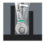
The Joker 6003 combination wrench with its special mouth geometry — an open-end offset by 7.5° and the double hexagon geometry — doubles the placement possibilities when repeatedly turning the wrench 180° around the longitudinal axis. Bolts and screw heads can be "accessed" every 15°. The Joker 6003 will automatically find the respective placement point after every turn.
