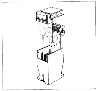
LDG-A-16 housings are capable of accomodating up to two lengthwise circuit boards in addition to one top circuit board as a crosswise connection and to accomodate any actuating and indicating elements.
