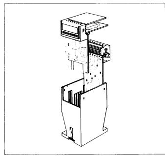
LDG-A-30 housings are capable of accomodating up to two lengthwise circuit boards in addition to one top circuit board as a crosswise connection and to accomodate any actuating and indicating elements.
