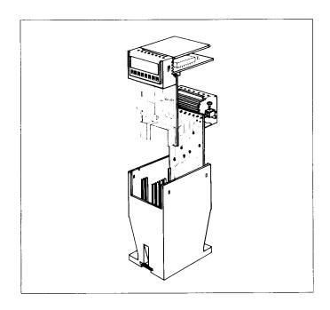
LDG-A-14 housings are capable of accomodating up to two lengthwise circuit boards in addition to one top circuit board as a crosswise connection and to accomodate any actuating and indicating elements.
