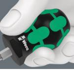
The 2-component Kraftform handle allows high power transmission due to the non-slip, softer grip areas and high working speeds due to the hard grip areas, which allow a guick hand switch.
