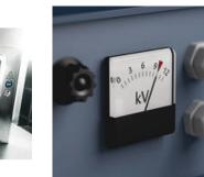
Our screwdrivers are tested for dielectric strength under a 10,000 volt load to make sure that their most important property, their insulation, has been exhaustively tested. Each individual Wera VDE screwdriver is subjected to this test to guarantee safe working up to 1,000 volts.
