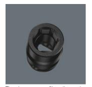
The hexagon profile allows the transmission of high forces and puts less strain on the edges of bolts or screw heads than a double hexagon profile. Fine-toothed ratchets also make the use of a double hexagon profile superfluous, even in confined spaces, thanks to their small backpivoting angle.
