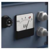
Our screwdrivers are tested for dielectric strength under a 10,000 volt load to make sure that their most important property, their insulation, has been exhaustively tested. Each individual Wera VDE screwdriver is subjected to this test to guarantee safe working up to 1,000 volts.
