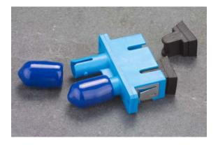
An optical fibre adapter or uniter is used to mate two connectors together, usually mounted in a distribution panel or wall box. In most cases it is the critical part of the system that aligns the ferrule part of the connectors keeping the fibres in perfect alignment.
