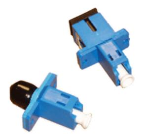
An optical fibre adapter or uniter is used to mate two connectors together, usually mounted in a distribution panel or wall box. In most cases it is the critical part of the system that aligns the ferrule part of the connectors keeping the fibres in perfect alignment.
