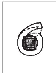
Too much „Pig Tail“: the last turn of connection is not formed against the terminal damaged wrapping bit ratio between terminal width and thickness too large
