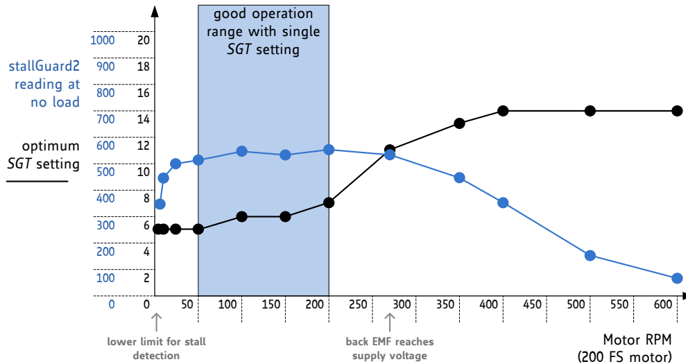
Figure 11.2 Example: Optimum SGT setting and stallGuard2 reading with an example motor
