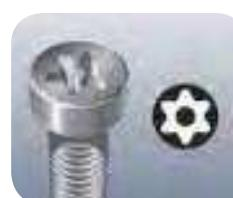
TORX® tools with a borehole prevent the unauthorised unfastening of safety screws. The screws contain a pin that protrudes into the drive profile so that "normal" TORX® tools cannot be used. This pin fits into the borehole of TORX® BO tools allowing safety screws to be unfastened.
