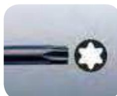
TORX® drive profiles transfers torque between tool and screw by parallel line or surface contact rather than point contact as many other profiles. This protects both the screw profile and the tool profile. It also increases the amount of torque and power that can be transferred.
