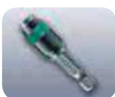
With the Wera Rapidaptor,  $\frac{1}{4}$ " bits can be inserted and automatically locked in the holder without using the slide switch. Even the smallest bits are easily removed by sliding the sleeve forward. The free-spinning outer sleeve stabilizes battery or mains-powered tools during the screwdriving process. All functions can be carried out with just one hand. There is no faster bit change!
