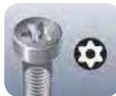
TORX® tools with a borehole prevent the unauthorized unfastening of safety screws. The screws contain a pin that protrudes into the drive profile so that "normal" TORX® tools cannot be used. This pin fits into the borehole of TORX® BO tools allowing safety screws to be unfastened.
