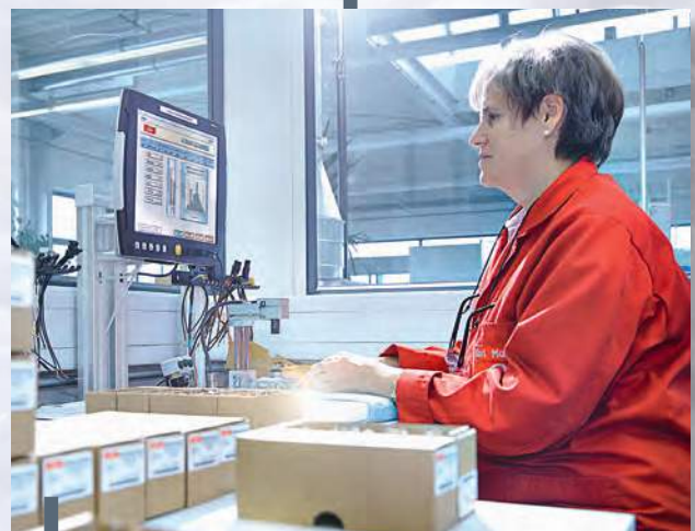
Fully automated switching point adjustment with computer-aided documentation of readings.
