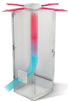
Hot air can also be expelled from the roof of the cabinet if, for instance, the sides of the cabinet are covered by obstacles, walls or by the sides of other cabinets. In a perfect configuration, an exhaust filter is positioned at the bottom of the cabinet.
