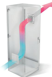
The use of exhaust filter ensures the passage of air and the removal of heat in a natural manner. This solution can be considered for dissipating low level of heat in dusty environments.
