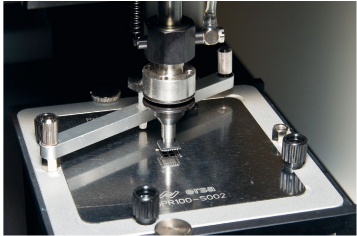
Component is lifted off the print stencil
