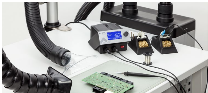
Fully equipped i-CON2 V workplace with i-CON2 V station, i-TOOL, CHIP TOOL VARIO and solder fume extraction
