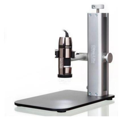
The Dino-Lite RK-10A is a sturdy and stable high-end stand solution that can be used with all the professional Dino-Lite models. It is constructed of resilient stainless steel and lightweight aluminum and offers a very precise fine-focus adjustment as well as a quick release function.
