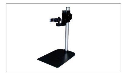
The AM35B is an economical and rigid vertical desktop stand that was designed to be used with the Dino-Lite handheld digital microscope cameras. It provides up to 360 degrees of horizontal axis rotational perspective and as much as 20cm of vertical working distance from the object.
