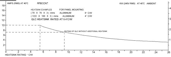
WITH HEATSINK RATING AS SPECIFIED THE MAXIMUM LOAD CURRENT CAN BE DETERMINED THIS IS THE MAXIMUM LOAD CURRENT POSSIBLE WITHOUT EXCEEDING THE DEVICE RATINGS
