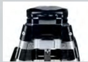
The 165 cm tall, ball-head tripod allows an AL 26 to be aligned rapidly.
