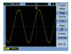
Normal sweep waits for a waveform that meets the trigger conditions before displaying any activity.
