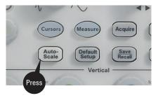
The oscilloscope analyzes all active channels, turning them on and setting the time base, V/div, and trigger conditions for an initial display.
