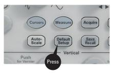
The oscilloscope is now set in the factory default configuration – just as it left the factory. Since the oscilloscope may have been used in a variety of applications by a variety of people, it is a good measurement procedure to put the oscilloscope in a known starting mode (Default Setup). This will make it easy to duplicate measurements as no special conditions will be set.
