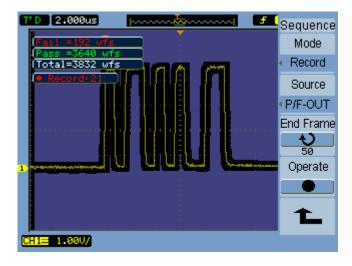
28 Press Operate again to stop recording waveforms.
