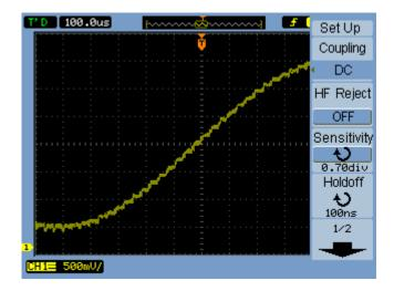
With the training kit board's noisy sine waveform, you can also turn on **HF Reject** to attenuate frequencies above 100 kHz. With the higher frequencies attenuated, the oscilloscope will trigger on the rising edge of the sine wave at the default sensitivity of 0.3 div.
