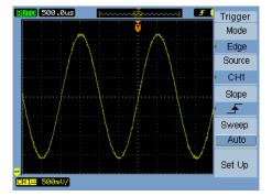
Auto sweep forces triggers if the trigger condition is not met and shows untriggered waveform activity.
