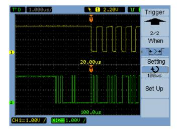
The channel 1 and channel 2 signals are captured using different triggers and displayed in different horizontal scales.
