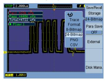
3 Press Internal to save to (or load from) one of the 10 internal storage locations, or press External to save to (or load from) a location on a USB drive.
