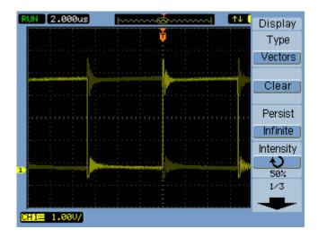
Being able to trigger on both edges of a waveform and use infinite persistence gives you a display similar to an eye diagram.
