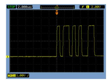
Note that "STOP" appears in the upper left corner of the display after the single acquisition has completed.
