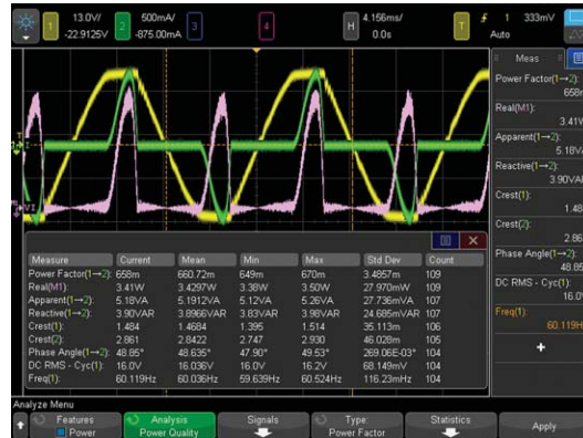
Figure 5 The power measurements option provides a results table with the following power quality measurements: Power Factor, Real Power, Apparent Power, Reactive Power, Crest Factor and Phase Angle.
