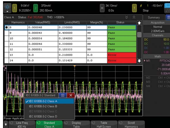
Figure 3 Perform the pre-compliance line harmonic testing of your power supply to the IEC 61000 3-2 standards. This analysis presents up to 40 harmonics.
