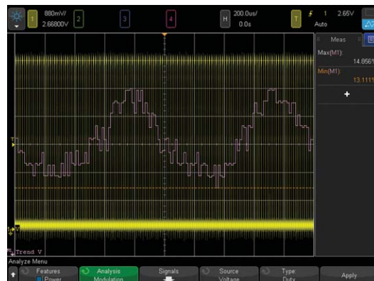
Figure 6 Plotting the embedded variation of on time or off time in the PWM signal over a long period of time can reveal the control loop response of the feedback loop system.
