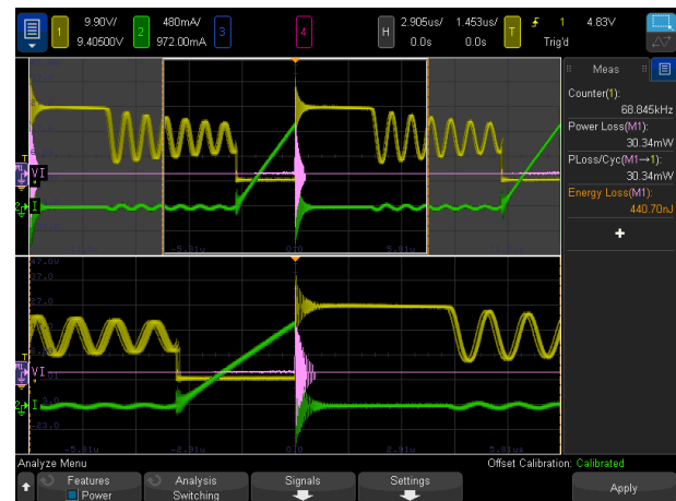
Figure 4: Switching loss measurement using the MSOX4154AUT power best bundle.
